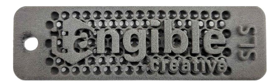
Selective Laser Sintering creates 3D prints by fusing layers of nylon powder. Because the powder acts as its own support, this method of 3D printing is ideal for parts with complex forms and drastic overhangs. As a result SLS 3D prints can be used for a wide variety of functional parts and has a textured finish.
