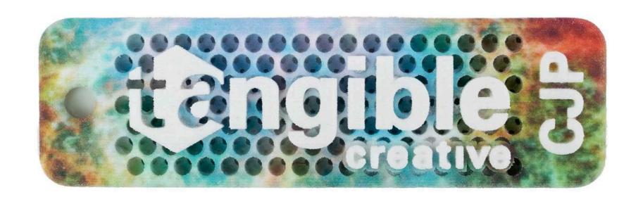
Color Jet Printing creates 3D prints using gypsum powder. Similar to the process of creating casts and objects with plaster, the CJP machine infuses the gypsum with an adhering glue and color pigments to create full spectrum colored 3D prints. The final texture is similar to SLS prints due to the powdery finish and texture. CJP prints can be coated in gloss or matte, to bring out the colors within the 3D prints.
